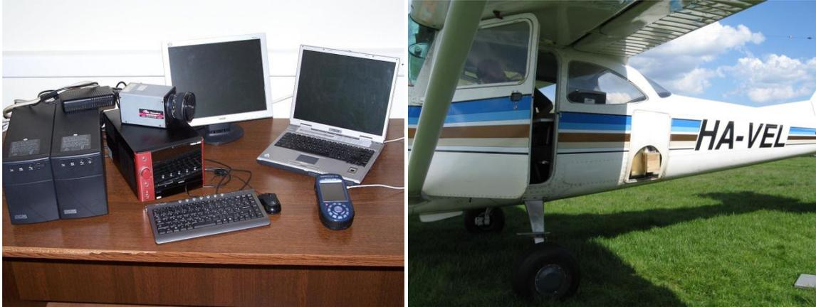
Fig. 1 Hardware elements of the recording system (left) and the Cessna 127 airplane with the CIR camera fixed into its luggage space (right)
