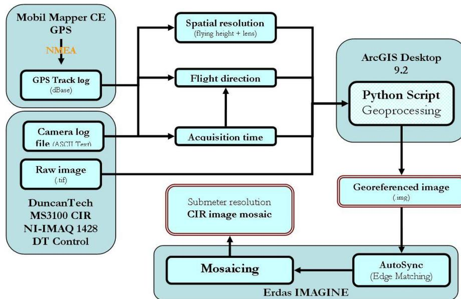
Fig. 5 Flow diagram of image processing from the raw images to the image mosaic
